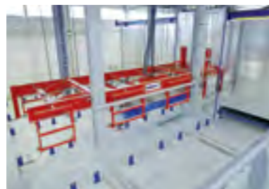
Vario STORE storage retrieval machine
